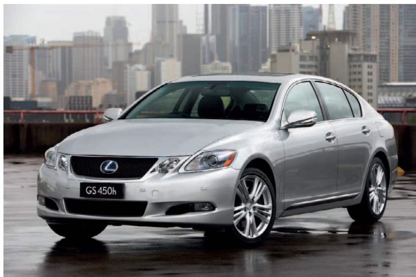
The Lexus GS 450h is powered by a 3.5 litre V6 petrol engine and permanent-magnet electric motor
