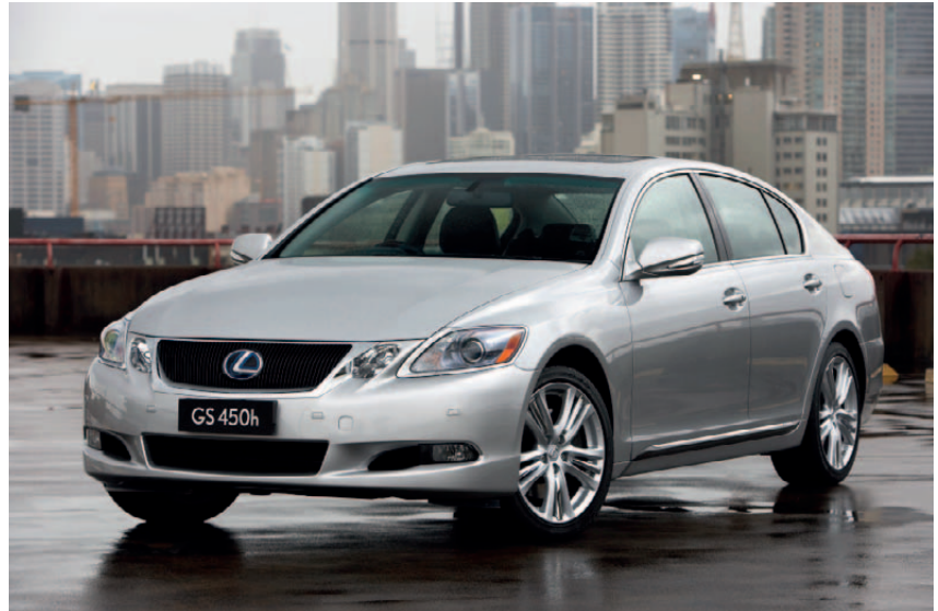
The Lexus GS 450h is powered by a 3.5 litre V6 petrol engine and permanent-magnet electric motor
